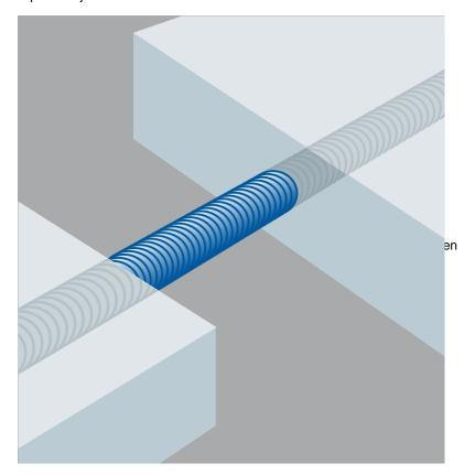
Corrugated polyethylene tubing is a good choice for protecting Myson PEX when crossing expansion joints.
